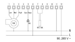
Wiring diagram for 4-pipe fan coil
