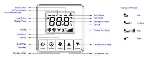
By pressing the MODE Button for more than 3 seconds, the parameter interface will appear.
